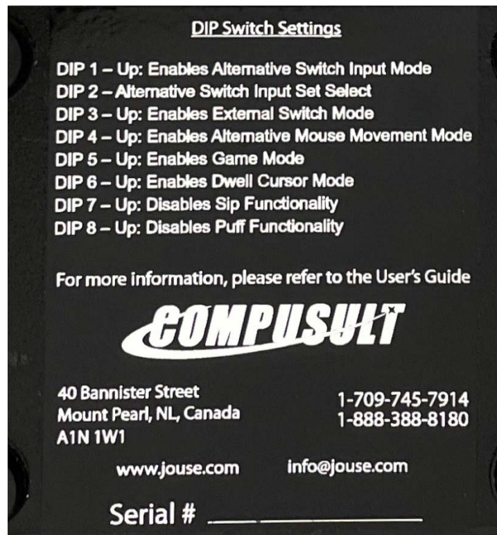
Figure 3-1: Jouse+ DIP Switch Settings
