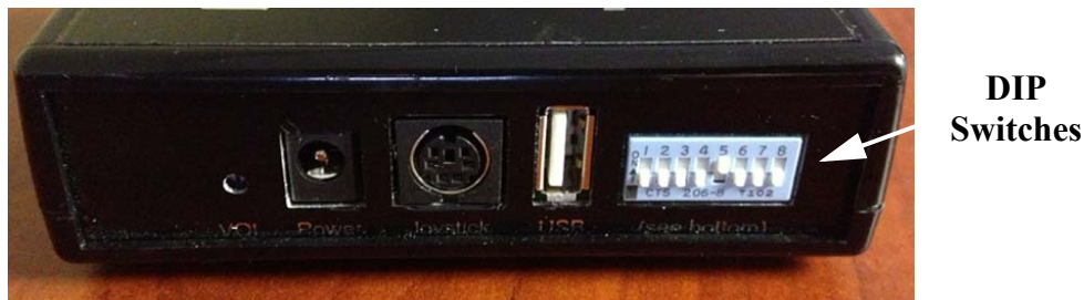
Figure 3-2: Jouse+ DIP Switches
