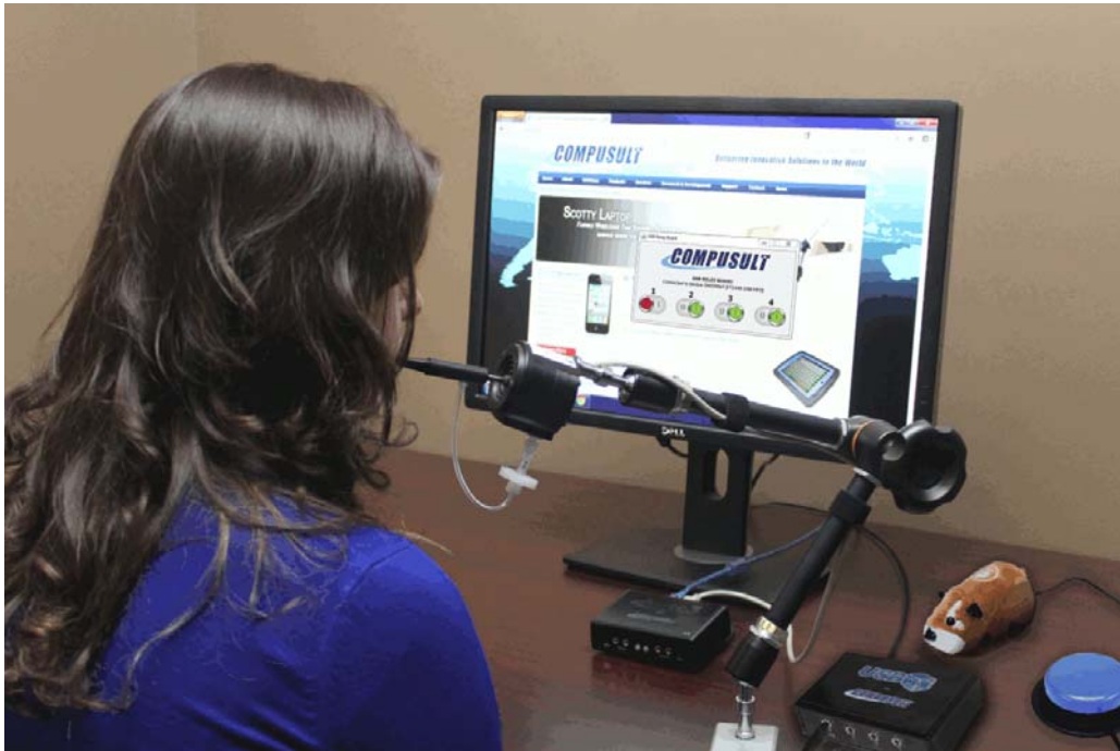
Figure 5-2: Jouse+ User Controlling a Switch-Enabled Toy Using the USBox Accessory
