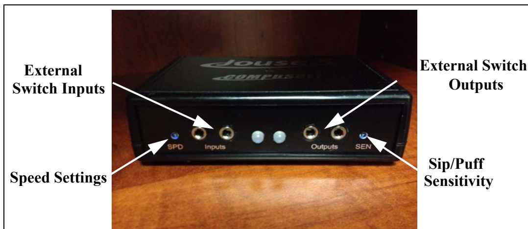
Figure 4-5: Jouse+ Front Potentiometers
