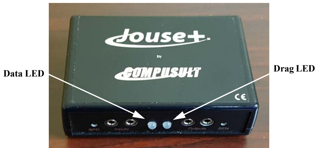
Figure 4-1: Jouse+ Indicator/Status LEDs
